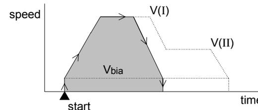
The PGU decelerates before reaching P(I) when the travel distance to decelerate to stop from V(I) is larger than P(II).
