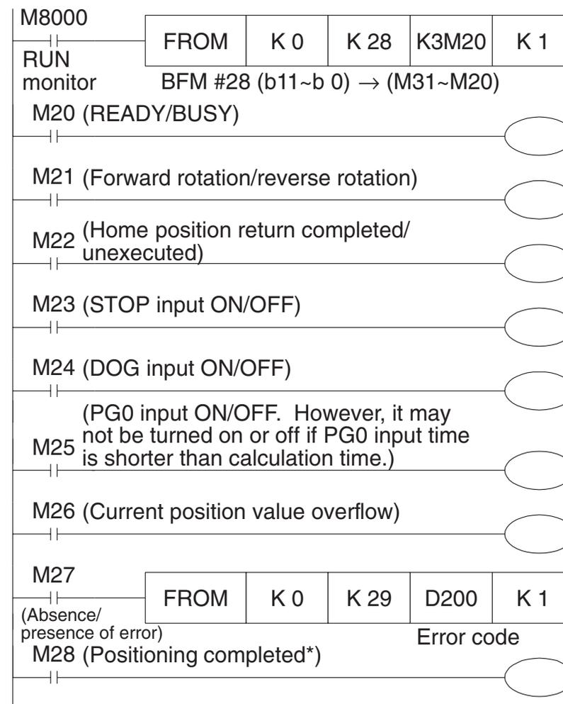
\* When a drive amplifier for a stepper motor without the positioning completed output is used, this signal can be used for recognition of positioning completed and the next operation can be started.
