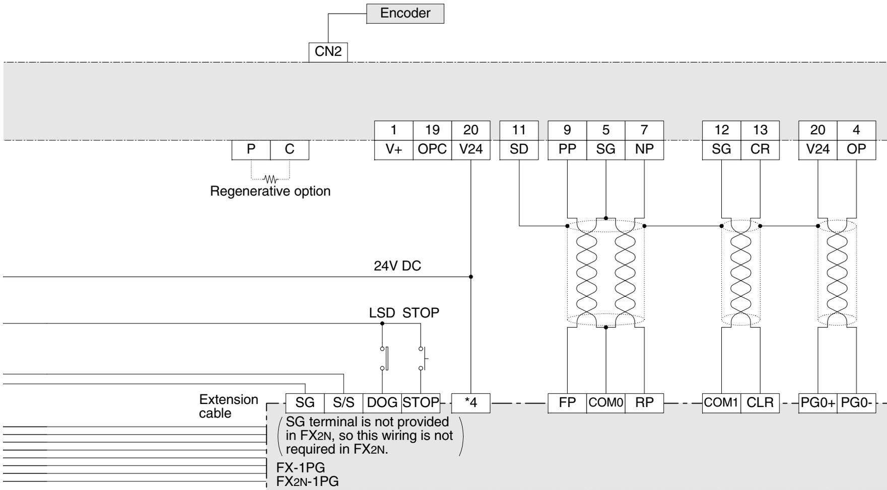
\*4 FX-1PG : Connect the VH terminal when the external power supply is 24V DC. Connect the VL terminal when the external power supply is 5V DC. Connect the FP0 and RP0 terminals with the Power Terminal for Pulse Output currently used.
