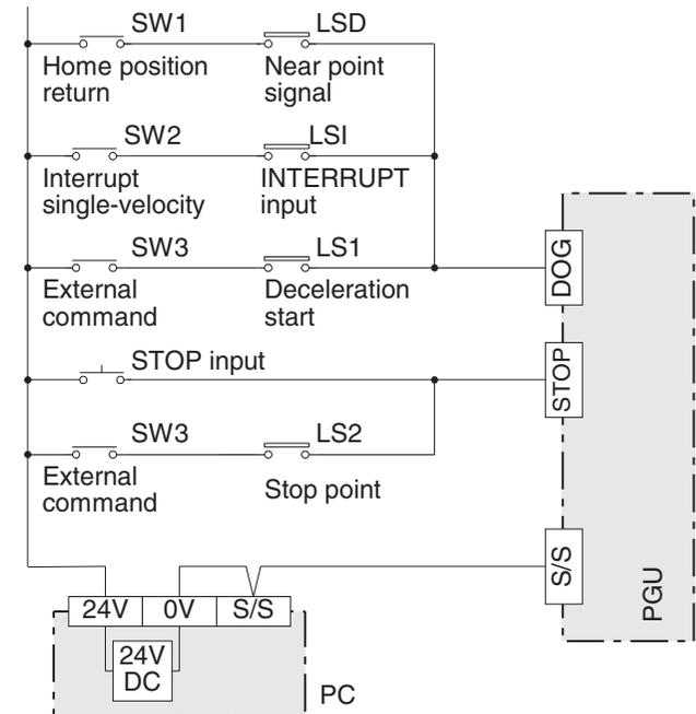
Input switches SW1 to SW3 are selected in accordance with the type of operation.
