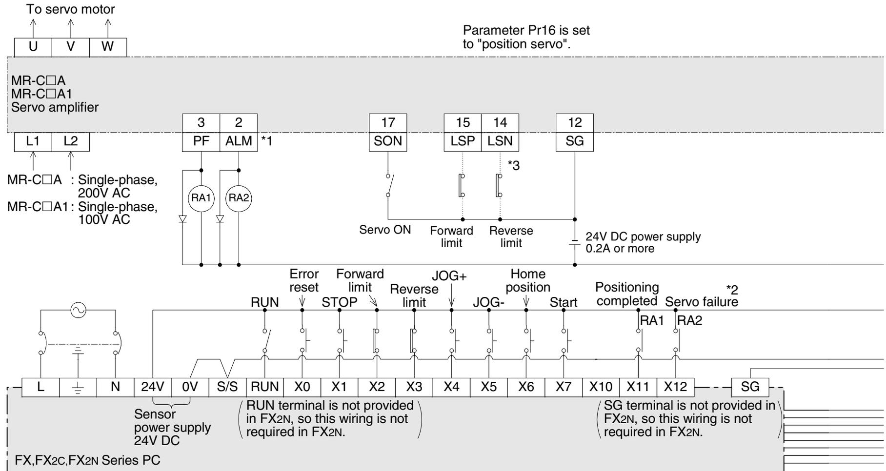
\*1 To release the alarm status, turn off the power, remove the cause of the alarm, then turn on the power again.
