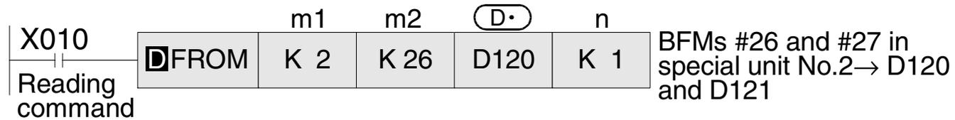
m1 : Special unit/block No. (K0 to K7 starting from the one nearest the basic unit)
