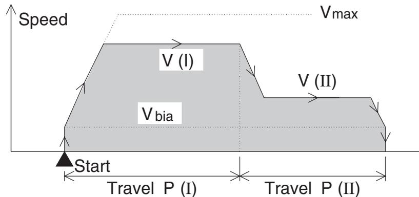
When the start command is received, the motor performs positioning at the operating speed  $V(I)$  (BFMs #20 and #19) until the set position  $P(I)$  (BFMs #18 and #17), then at the operating speed  $V(II)$  (BFMs #24 and #23) until the set position  $P(II)$  (BFMs #22 and #21) (two-step speed).
