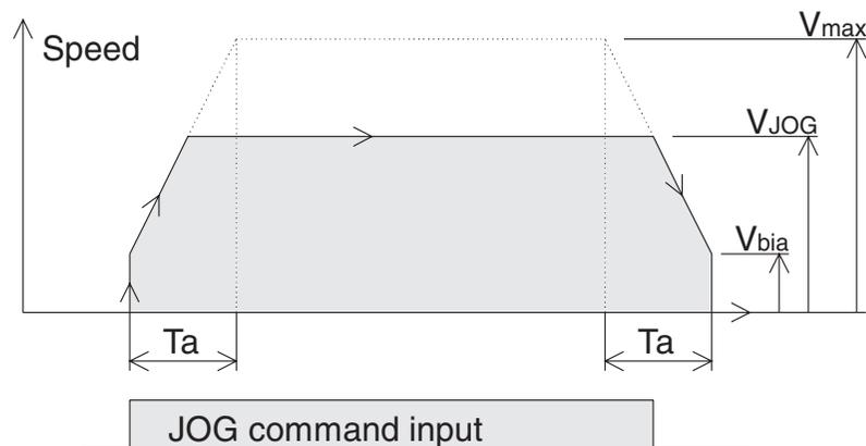
Any value between the bias speed  $V_{bia}$  (BFM #6) and the maximum speed  $V_{max}$  (BFMs #5 and #4) is valid as the command speed  $V_{JOG}$  (BFMs #8 and #7). The acceleration/deceleration time  $T_a$  (BFM #15) is the time between  $V_{bia}$  and  $V_{max}$ .
