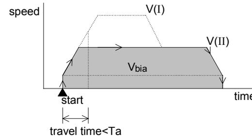
If the travel time is shorter than the time ( $T_a$ ) for the PGU to accelerate to the operation speed I, the PGU operates at the operation speed II from the beginning.
