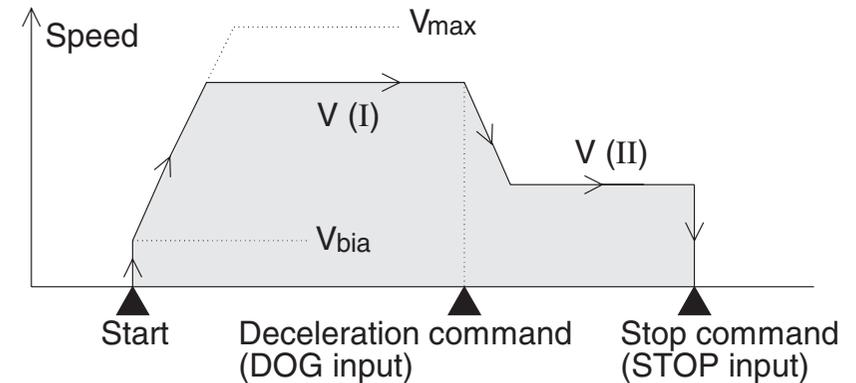
When the start command is received, the motor performs positioning at the operating speed  $V(I)$  (BFMs #20 and #19) until the deceleration command is received. At that time, the motor decelerates to the operating speed  $V(II)$  (BFMs #24 and #23). When the stop command is received, pulse generation is stopped immediately.
